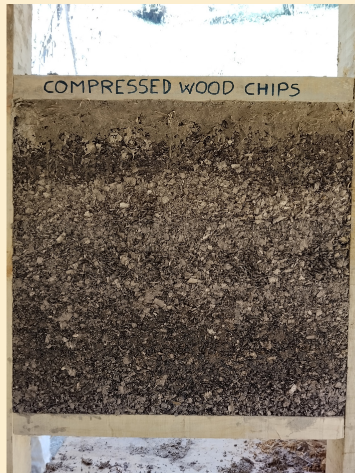
Light clay with wood chips
