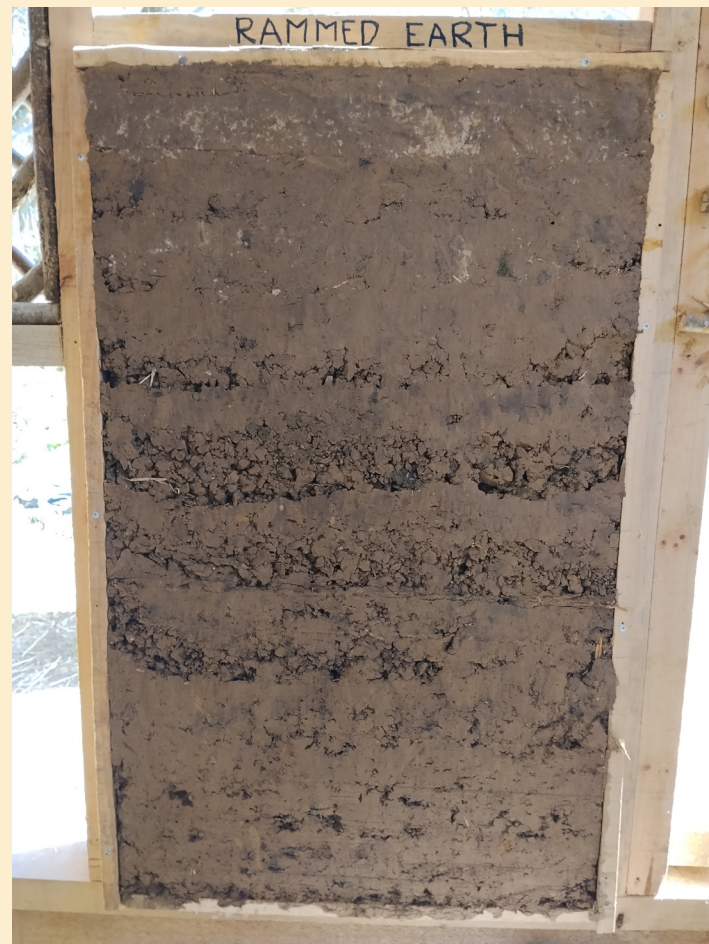
Rammed earth with darker clay
